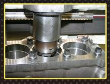
For the best possible cylinder wall geometry, JASPER utilizes Torque Plate Boring and Honing with a torque plate and speciallydesigned ARP2000\* head bolts.
