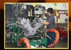
JASPER Engines undergo Live-Run Testing using state-of-the-art Data Acquisition to check compression, vacuum and oil pressure to assure reliability.
