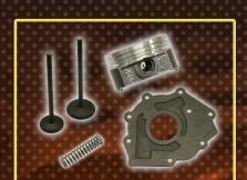
JASPER upgrades 4.6/5.4/6.8 engines with nitrided valves, JASPER designed pistons and, on 3-valve VVT V8 engines, a high-volume oil pump with a higher pressure relief valve spring and updated backing plate to improve durability and operation.
