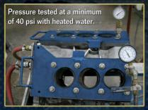
JASPER 100% pressure tests the coolant passages on GM 3.6L blocks to ensure there are no cracks or leaks.
