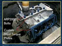
For the best possible cylinder wall geometry, JASPER torque-plate hones all GM 3.6L GDI blocks to ensure the bore is consistent from top to bottom for improved ring sealing, and reduced piston scuffing and oil blow-by.
