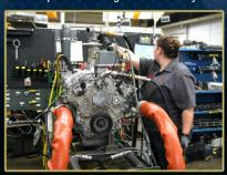
JASPER Engines undergo Live-Run Testing using state-of-the-art Data Acquisition to check compression, vacuum and oil pressure with other assessments for your assurance of reliability.
