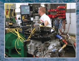
Every remanufactured engine from Jasper Marine is tested before it leaves the factory. Popular Complete Engines are live-run tested with recorded inspections on compression, vacuum and oil pressure readings. Complete Engines are also checked for proper lubrication to the rocker assemblies, and black-light tested for leaks.
