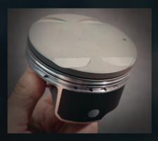
An accumulator groove is machined into the piston to decrease the pressure between the 1st and 2nd ring land, preventing the upper (compression) ring from unseating at higher RPMs.
