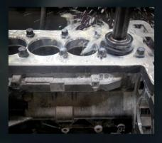
100% torque plate honing, utilizing a torque plate and ARP2000® bolts, provides cylinder wall geometry that matches the cylinder head as a complete running assembly, for improved ring sealing. (See picture above.)
