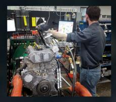
100% Live-Run Tested, utilizing Data Acquisition with other assessments for your assurance of reliability. These tests include: compression, vacuum, oil pressure, actuator and reluctor testing, and blacklight leak testing.
