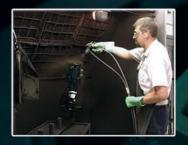
JASPER Sterndrives and Lower Units undergo a special nine-step paint process, which includes an oven-baked finish for ultimate protection from the elements. Lower Units are pressure and gear tolerance tested to ensure smooth operation and optimum performance.
