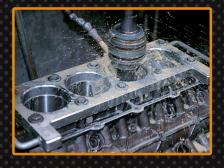
For the best possible cylinder wall geometry, JASPER torque-plate hones all Chrysler 5.7L Hemi blocks to ensure the bore is consistent from top to bottom.
