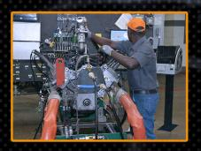
JASPER Engines undergo Live-Run Testing using state-of-the-art Data Acquisition to check compression, vacuum and oil pressure for your assurance of reliability.
